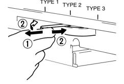
Slide the Lens Unit into the machine along the Lens Guide.
